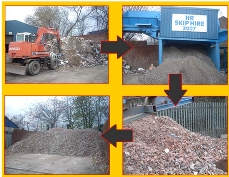
Photo. 4 Bricks recycling plant ( HR skip hire ).
